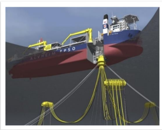
Internal turret single-point mooring system
